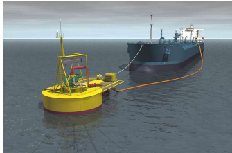
Conventional tanker connecting directly to calm buoy.
