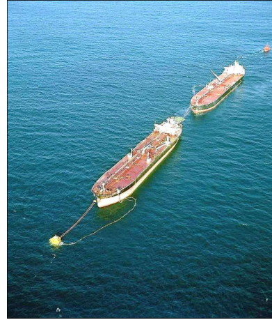
FSO permanently connected to calm buoy
