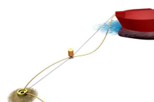
Single anchor loading SAL
